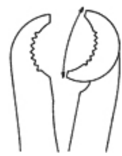
IM-11-1215-27 Lambotte 27cm 10 3/4" Bone Holding Forceps one flexible jaw
