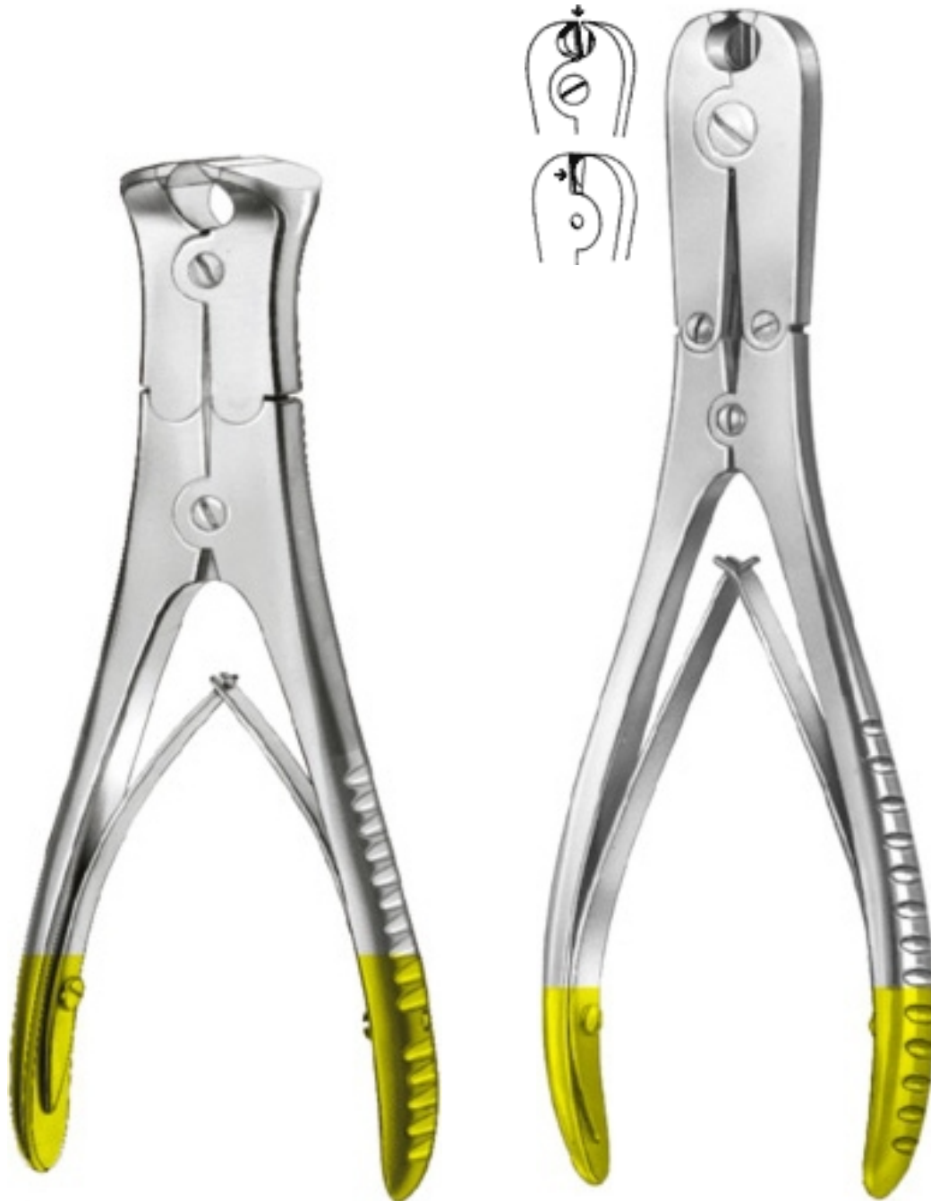
MI-11-320-15 6" Wire Cutting Pliers for soft wires up to 2,0 mm Ø for hard wires up to 1,2 mm Ø
