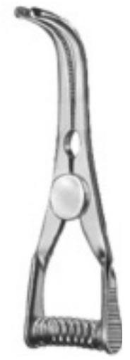
Bulldog Clamp IM-03-480-35 35 jaw length 14 mm closing pressure 220 +/- 10 gr.weight 1 gr.
