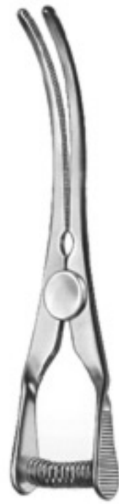
Bulldog Clamp IM-03-465-50 50 jaw length 21 mm closing pressure 110 +/- 10 gr. weight 1,5 gr.
