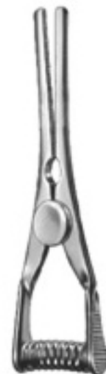
Bulldog Clamp IM-03-460-35 35 jaw length 13 mm closing pressure 110 +/- 10 grweight 1 gr
